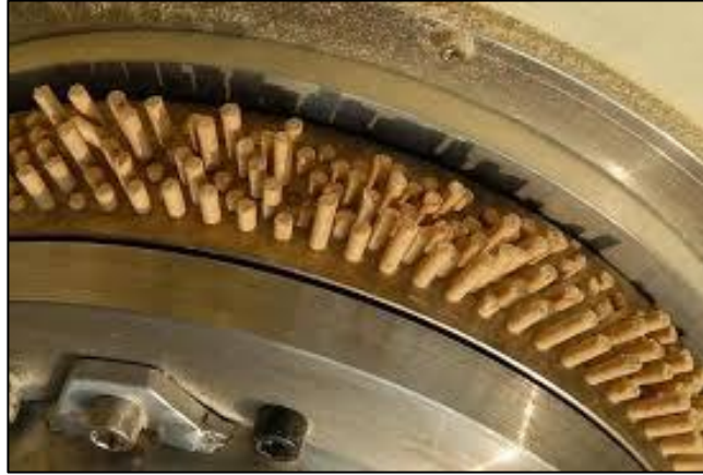
Figure 3.1: Wood pellet were produced from pelletizer.
